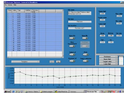
Thickness, EC 02. Performs thickness measurements and calculations of compression set. Can be connected to Mitutoyo gauges, for example.
