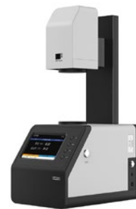
A haze-meter measures several transparency parameters in one instrument: total transmission and haze.
