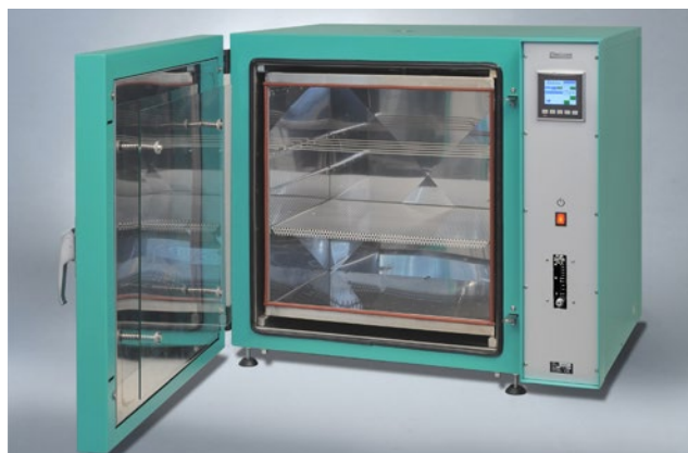
Cabinet ageing oven EB 04-II has low air speed and a flow meter that can be set between 3 to 20 changes per hour, which meets the requirements in ISO 188 method A.
