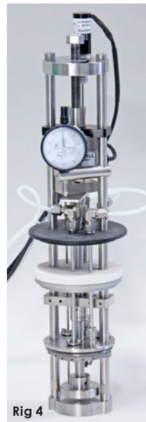
Rig 4 is arranged for testing according to ALE test.
