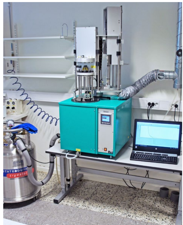
Combined low temperature instrument with a Gehman tester (ET 02-II) selected, placed on the adjustable table ET 01.08.
