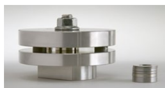
Compression set rig, EV 03.
