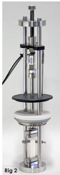
Rig 2 is arranged for testing in tension according to ISO 6914 method A.
