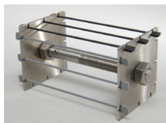
Tension set rig, EV 04.
